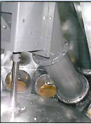
Brush on Swing Spout to Reduce Dust Buildup
