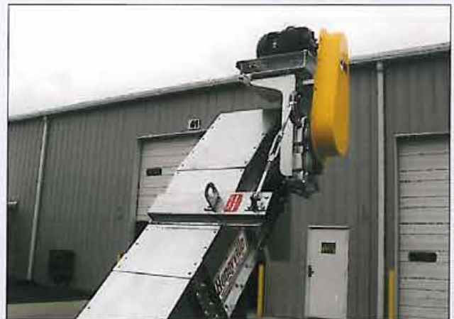
Top Mounted Torque Arm Gear Box Drive w/Motor Mount
