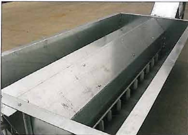
Smooth Self-Cleaning Slopes Inside Pit Hopper
